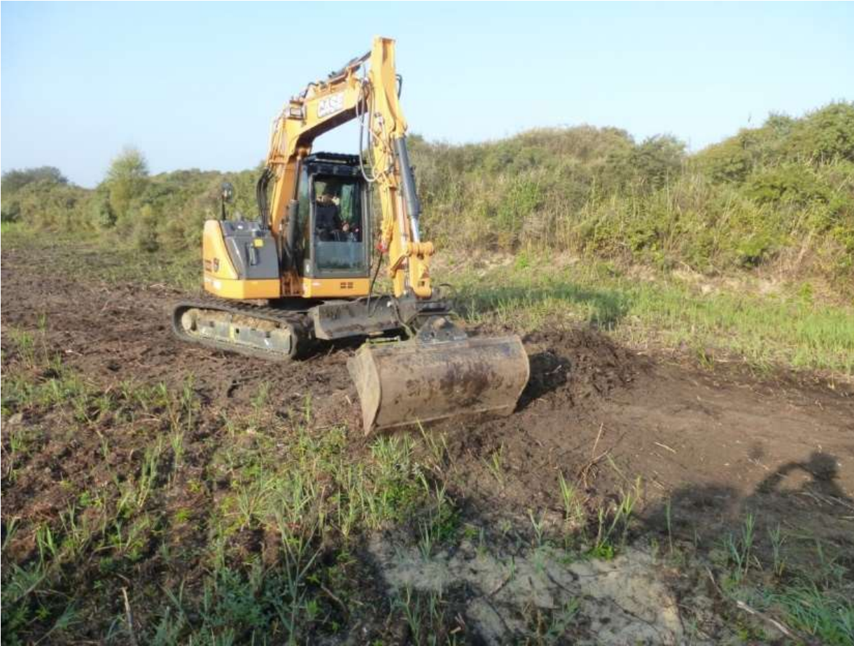
Photo: 'De Westhoek': restoration of an ancient humid dune slack by removal of scrub followed by cutting off sods.
